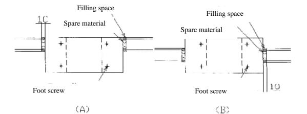
③ Processing for fixing bottom of the body
