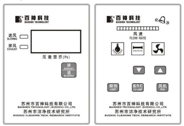
5.1 Turn on the power supply: insert the power cord plug into the socket of the equipment rear, insert another end to the power socket, open the switch with the key, the screen of differential pressure turns to red, indicate the power is on.
